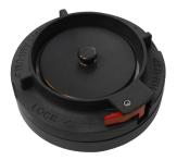
Mueller also offers latching and non-latching 5" Storz adaptors for connection to 4-1/2" NST nozzles. Mueller Storz adaptors feature the same caps used on the integral Storz nozzle and meet the requirements of NFPA 1963. Mueller Storz adaptors are rated for 250 psi operating pressure.
